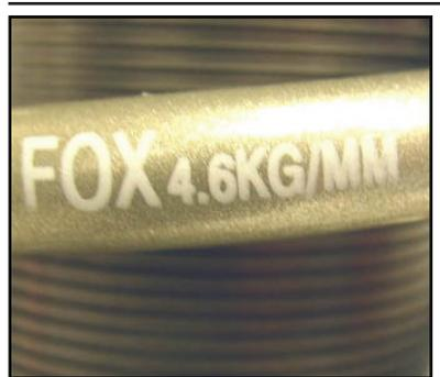
The spring rate is printed directly on the FOX shock spring.
