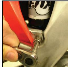
3. Remove the lower and upper shock mounting nuts and bolt and remove the stock shock.
