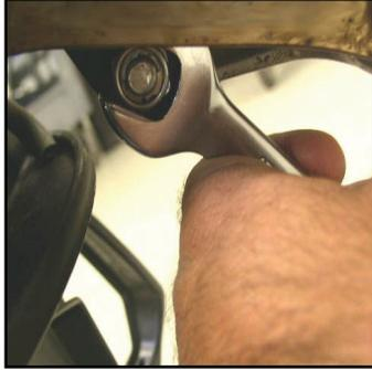
4. Double check the pre-installed upper and lower spherical bearing and reducers to your stock shock (to insure you have proper fit).
